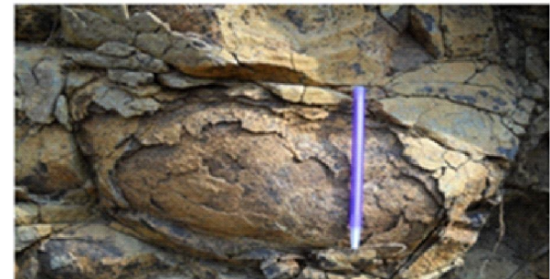
Fig. 10: Highly weathered basalt and exhibiting spheroidal weathering in basaltic rock observed near Jamkhar village
